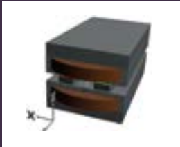
Simplified drawing of the Moving Magnet Motor
